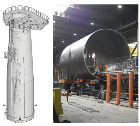
Left: 3D drawing of transition piece for wind turbine foundation. Right: The first transition piece is being manufactured. The transition piece consists of steel plates which are rolled and welded together.
